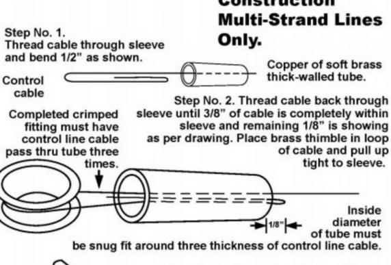
Step No. 3. Crimp sleeve in two places as shown in drawing. Use round-jawed long nose pliers. Note: This method of assembly not to be used on single-strand control
